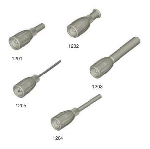
These adaptors can replace the Omnifit cap on any 'Omnifit Cap' connector or valve to give either quick push-on connections for softwall tubing or luer connections. Cap-to-luer adaptors are available with male or female luer connections. Cap-to-pipe adaptors are available in Tefzel® or stainless steel to accept softwall tubing with the following internal diameters: 1/16", 1/8" and 1/4".
